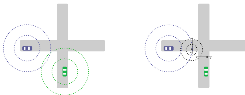
Exchange of data: vehicle-to-vehicle communication (V2V) (left) and vehicle-to-infrastructure communication (V2I) (right)
